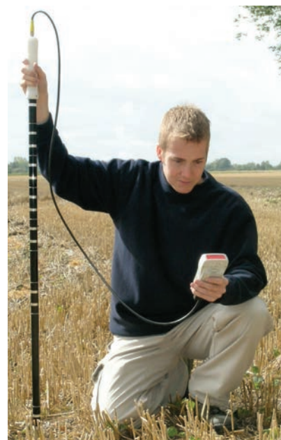
(Above) PR2/6 Profile Probe with HH2 Moisture Meter. (Right) PR2/4 Profile Probe
