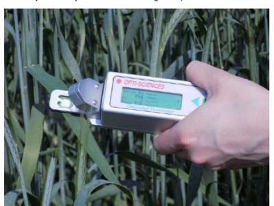
A compact and affordable light adapted Y(II) & ETR meter Quantum Yield of PSII or Y (II) is a test that allows the measurement of the efficiency of Photosystem II under actual light adapted
