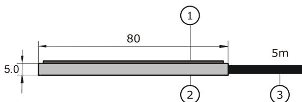
Figure 3 HFP01SC dimensions: heater (1) heat flux sensor body (2), cable (3)
