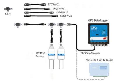
One WET150 can be read with a WET150 Meter. Multiple WET150s need a GP2 or other SDI-12 controller.
