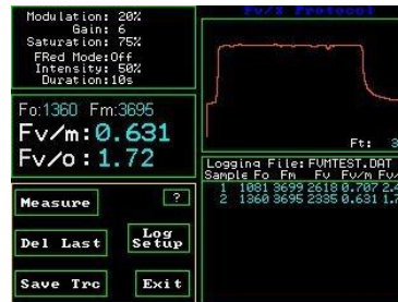
F_v/F_m measuring screen F_v/F_m F_v/F_o F_o F_m
