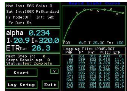
Rapid light curve measuring screen
