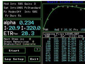
Quenching relaxation measuring screen measuring q_E , q_Z & q_I
