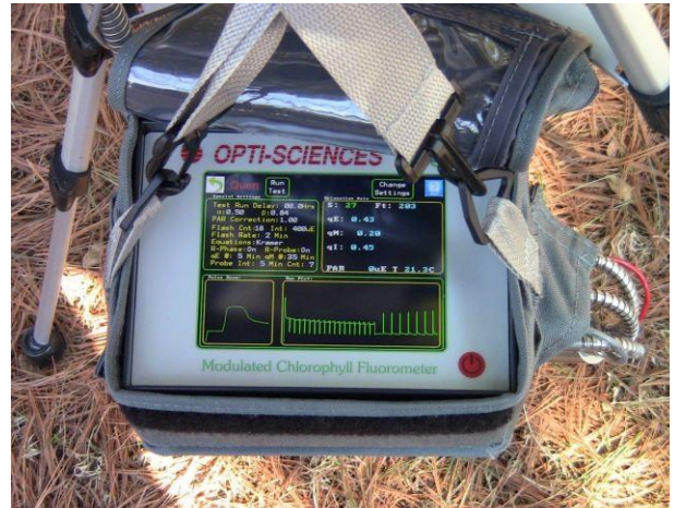
Quenching relaxation measuring screen measuring q_E , q_Z & q_I
