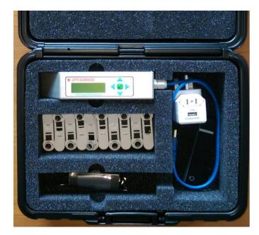
The Fv/Fm meter is supplied in a rigid, clam shell case which holds the meter, travel charger, battery, 10 dark adaption clips, charging lead and manual on a USB stick.
