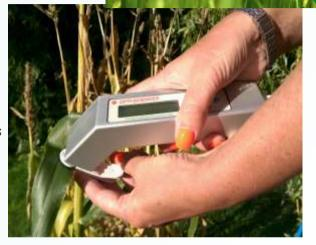
The measurements of Fv/Fm can be made in under 2 seconds.
